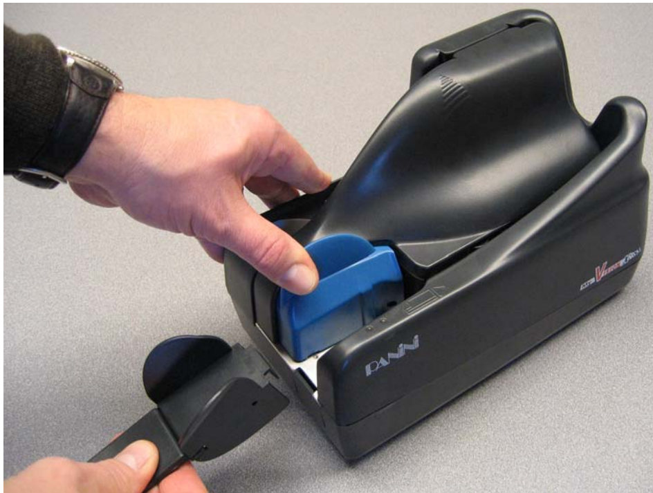
Figure 5: Installing the check feeder on a Panini MyVisionX scanner
