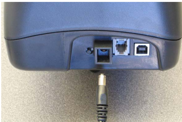
Figure 3: Plugging the power supply into the scanner
